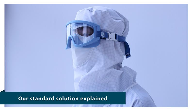
The most common solution is to attach the goggles directly to the coveralls. However, we have now developed a new and innovative solution which consists of attaching a textile strap directly to the goggles. These innovations were tested and validated and not only do they increase wearing comfort, they also significantly reduce CFU\* around the goggles.
